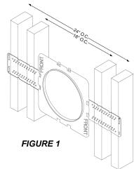
vide drywall Installers the correct cut-out pattern for the speakers. The mounting rings have "flaps" that nailed/screwed/ are stapled onto the joist. See figure 1. Once the wall board is installed, the opening is cut out to mount the speaker.
